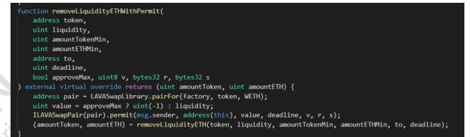
Figure 16 Source code of *removeLiquidityETHWithPermit*
